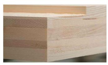
thickness varying between 17 and 40 mm, arranged orthogonally and glued with formaldehyde-free adhesives. The available thicknesses range from 51 mm to 320 mm, with maximum dimensions of 3.5 meters in width and 13.5 meters in length. The wood used belongs to the minimum strength class C24 and comes from sustainably managed forests, certified according to PEFC standards, prioritizing local sources to reduce environmental impact.
